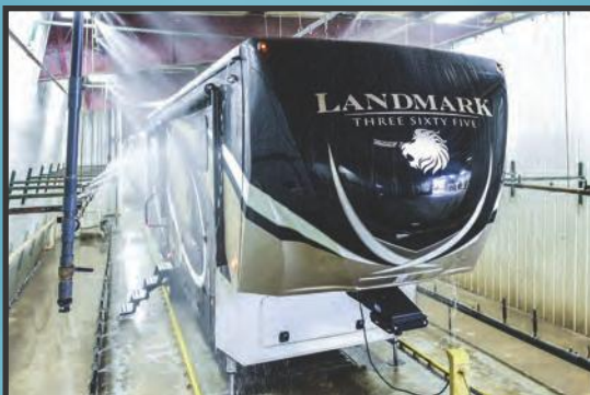
127 SPRINKLER RAIN BAY TEST
